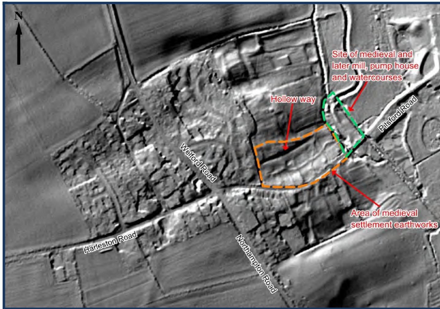
Figure 4: Terrain model of Chapel Brampton produced from Lidar data (© Environment Agency 2019) showing the medieval hollow way, settlement earthworks and mill site.
